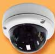
Domo color antivandálico Día/Noche CCD SONY Super HAD 560 TVL - 0,00001Lux Wide Lente varifocal aspherical 3,7/12mm Wide Dynamic Range (WDR) Sense Up - OSD High Spot BLC 3D Digital Noise Reduction
