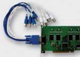
Placa digitalizadora 16 can. 100 CPS y 4 can. audio, 4 can. video, 100 CPS.
