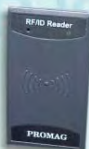
Lector Mifare ABA-WIEGAND-RS232 LED - BUZZER alcance 2-5 cm
